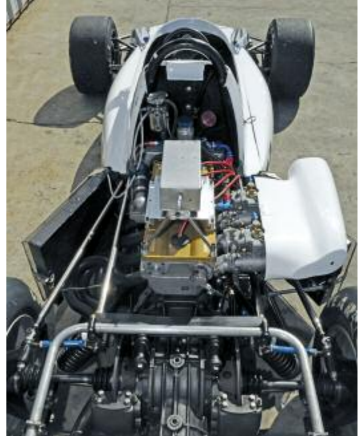
(Above) A tubular steel subframe bolts to the back of the March monocoque to cradle the engine, while fuel tankage required only small bulges in the bodywork on either side of the cockpit. Twin Weber DCOE carburetors were a requisite component of the standard Atlantic power-producing kit. (Below) Clutter apparent in rear suspension layout is evidence that back-half aerodynamics had yet to become a primary concern in Atlantic. (Bottom) The original March corporate logo employed a brand-new computer-recognition font called Data 70 to represent the four-man company's futuristic, forward-thinking mission.
