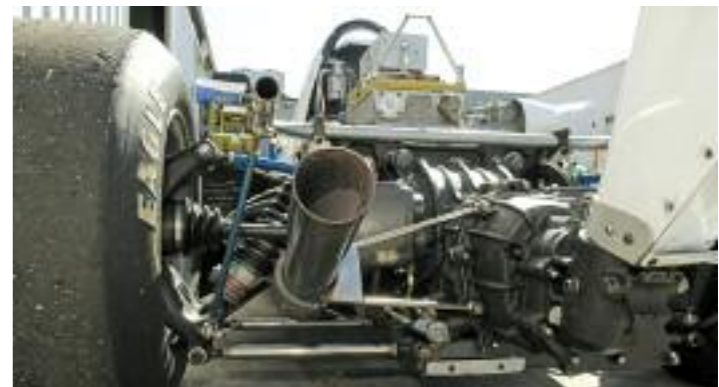
(Above) A tubular steel subframe bolts to the back of the March monocoque to cradle the engine, while fuel tankage required only small bulges in the bodywork on either side of the cockpit. Twin Weber DCOE carburetors were a requisite component of the standard Atlantic power-producing kit. (Below) Clutter apparent in rear suspension layout is evidence that back-half aerodynamics had yet to become a primary concern in Atlantic. (Bottom) The original March corporate logo employed a brand-new computer-recognition font called Data 70 to represent the four-man company's futuristic, forward-thinking mission.
